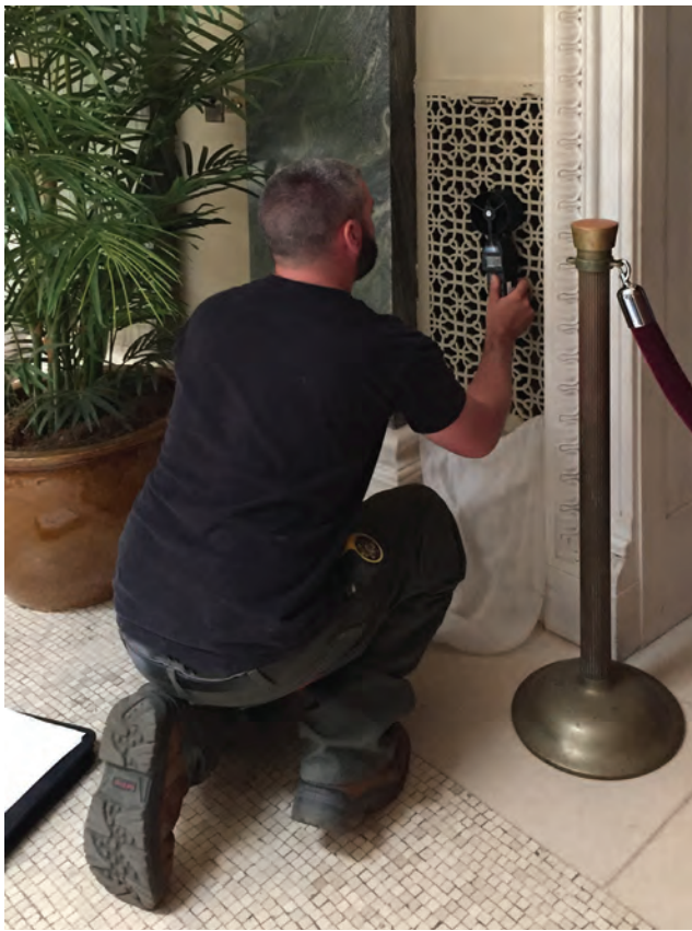
FIGURE 12 (left). Measuring discharge rates with anemometer and flow hood (right). LEFT: DAVID BITTERMANN RIGHT: MARGARET BREUKER, HACE
