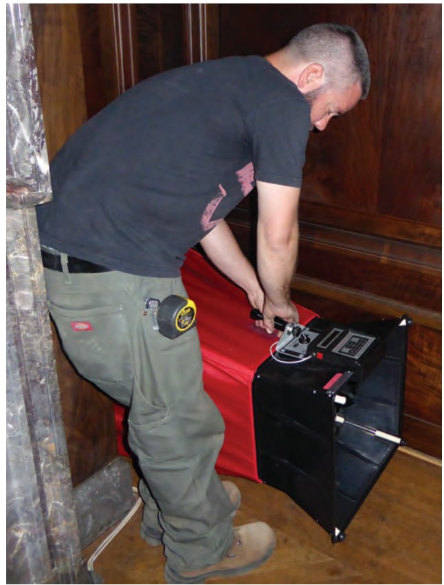
FIGURE 12 (left). Measuring discharge rates with anemometer and flow hood (right). LEFT: DAVID BITTERMANN RIGHT: MARGARET BREUKER, HACE
