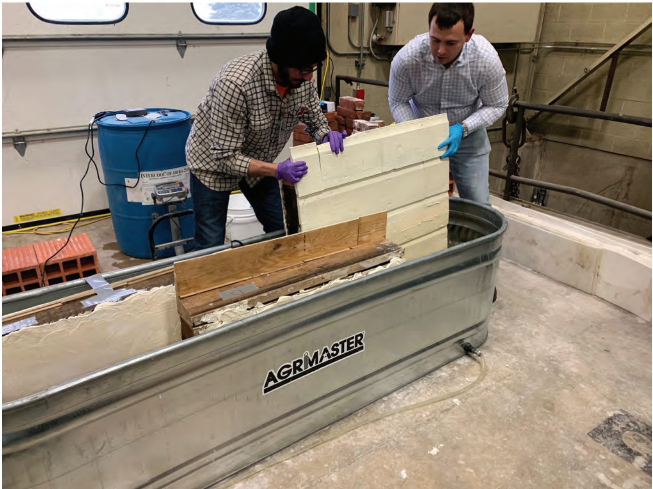
FIGURE 3. The Cultural Resources Partnerships and Science Directorate is collaborating with the US Army Corps of Engineers Engineer Research and Development Center to devise and implement a methodology for testing the flood resilience of historic building assemblies, materials, and finishes and substrates. NATIONAL PARK SERVICE
